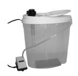
This handy etching tank system will handle P.C. boards up to 8" x 9" and 2 at a time. The tank holds 1.35 gallons of etching solution. The system is supplied with air pump for etchant agitation, heater for keeping etchant at optimum temperature and convenient board holder. Tank has tight fitting top to prevent evaporation when not in use. **No. 12-700**
